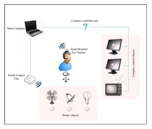
The head mounted eye tracker system with two small cameras will be carried by user and it can also be wirelessly in ideal case.
